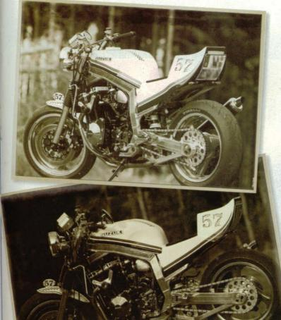
subframe off to replace it with something else, but in the cold light of day he realised that an Egli tailpiece fitted to a modified version of the original subframe would look best, so welded it back on again!
